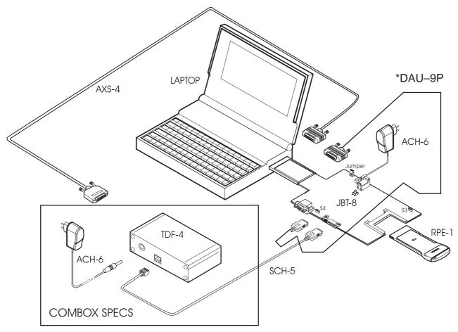
\*Note: If you want to operate only using Wintesla to do tunings etc., you just need to connect the DAU–9P from the PC serial port to the bottom connector of the JBT–8.
