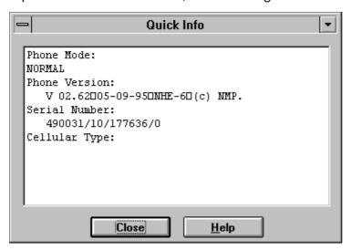
**Note!** Special conditions (For example, if the phone's SIM lock is ON) cause this dialog box to change color to make this special condition clear to the user.
